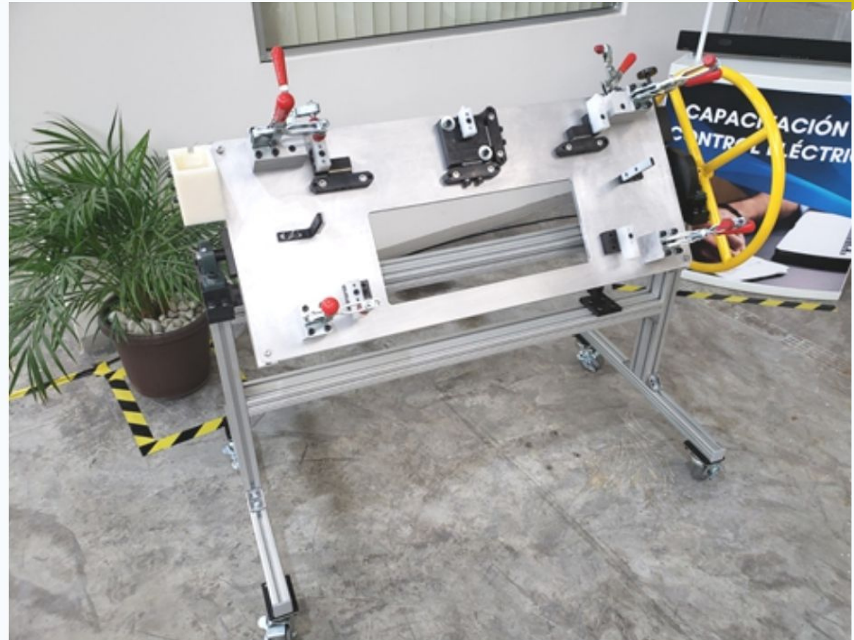
Manual assembly station
